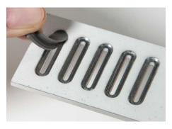
APS uses silicone masks to protect parts during plasma spray coating. APS has found that certain silicone formulations will yield 3D-printed masks that can withstand sandblasting and plasma spraying with satisfactory durability. These silicone-printed masks also have the advantage of being easily fitted and removed, while guaranteeing the precise boundaries and positioning of the masked areas on the parts.
