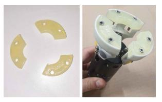
incompatible with the new bottle caps and had become worn: new non-slip, silicone jaws for the screwing tool.
